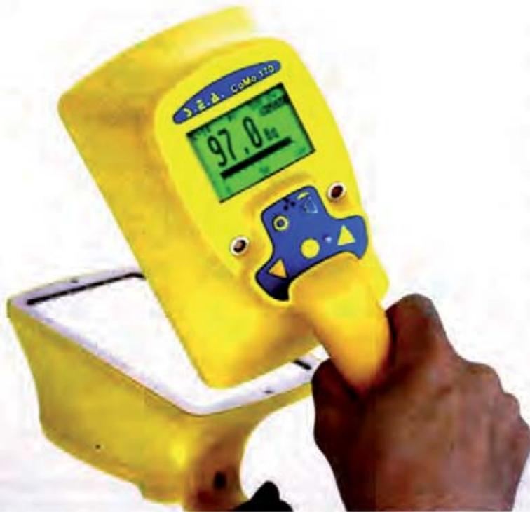
Abb. 1: Mobiler Kontaminationsmonitor CoMo-170
