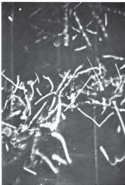
Figure 3. Cloud chamber photograph with many  $\alpha$ -tracks.
