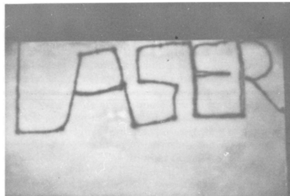
Figure 3. ZnS screen after UV excitation and subsequent irradiation with He-Ne gas laser. Dark lines forming "LASER" represent trace of laser beam on the screen.
