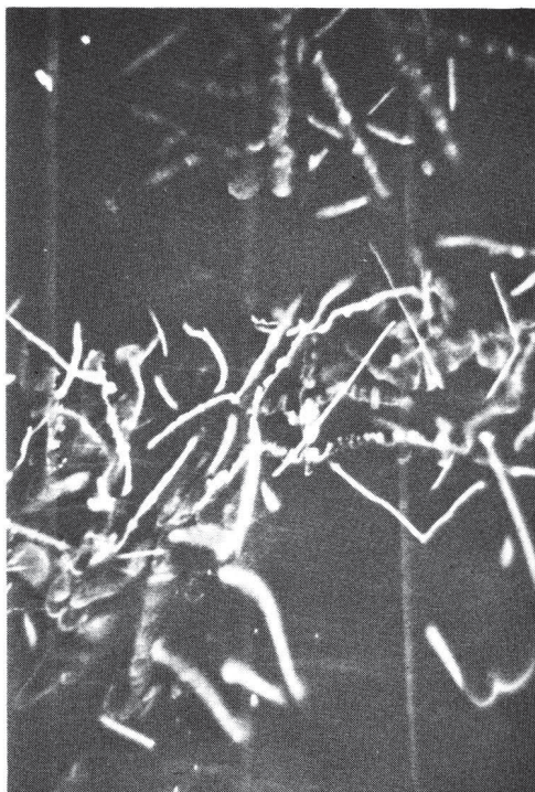
Figure 3. Cloud chamber photograph with many \alpha -tracks.
